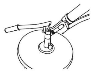
Start the unit and fill the small tank. Filling mayresult in the coupling rod being forced out of the lubricator line.
