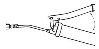
Lubricate by controlling the hand wand.
