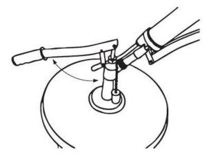
Pull the connecting rod to activate the jaw and slide the connecting rod back into the handle body.
